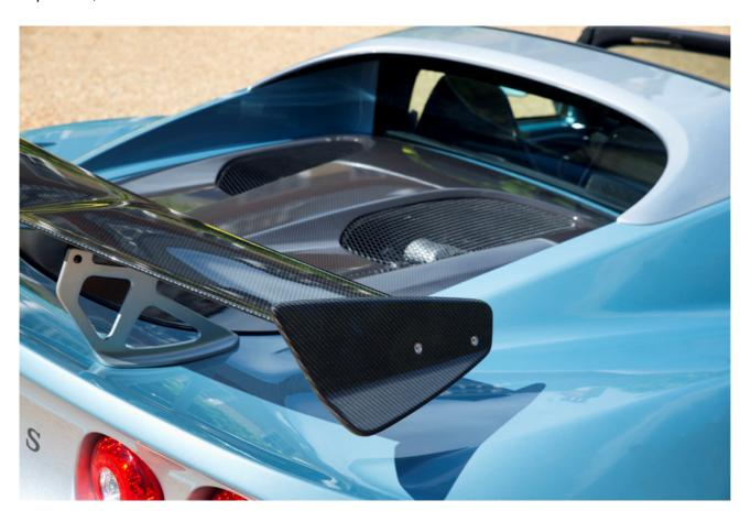
Powered by a high-output, supercharged, 1.8-litre 4-cylinder engine, the Elise 250 Special Edition boasts 243 hp (246 PS) at 7200 rpm and 250 Nm of torque between 3500 rpm and 5500 rpm. This, along with the car's 899kg kerb weight, contributes to the impressive 270 hp/tonne headline figure.
