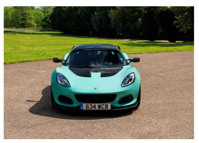
The Elise Cup 250 also includes a number of high-performance additions unique to this model. These include revised dampers and ultra-lightweight forged wheels with Yokohama Advan A048 LTS tyres - 225/45 ZR17 at the rear and 195/50 ZR16 at the front.
